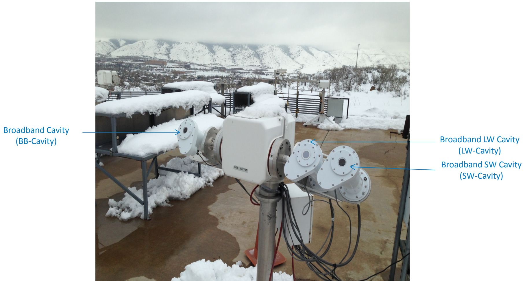
Calibrated five SW radiometers using SW-Cavity and BB-Cavity
