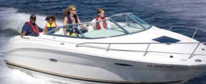
Woman at the helm of a motorboat wearing an inflatable belt pack with kill switch, with a girl passenger wearing a children's life jacket and an adult male and female wearing inflatable life jackets.
