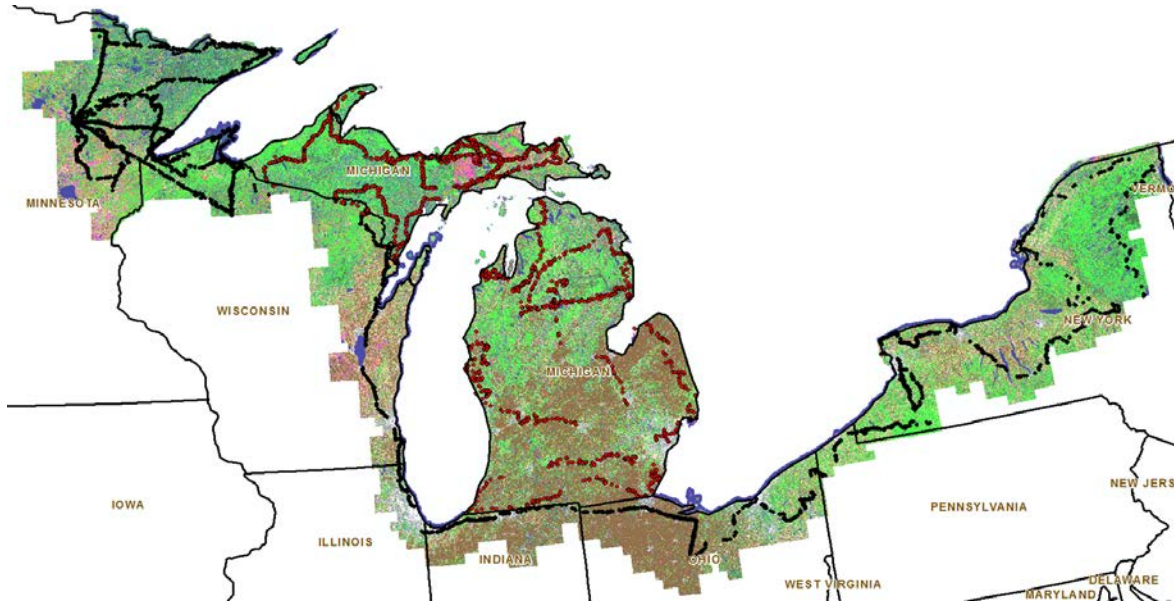
Figure 2. Accuracy assessment locations for the 2001 C-CAP Great Lakes area draped on 2001 land cover. Two accuracy assessments were performed for this region and are displayed as separate colors (red for Michigan, black for the remaining area of the Great Lakes C-CAP region). Sampling along road networks can be seen, along with clustering of sample locations (e.g., Grand Rapids, Minnesota, in the northwestern portion of the map).
