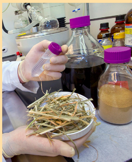
One-Pot Process. The right combination of enzyme cocktail and ionic liquid pretreatment can be used to extract fermentable sugars from switchgrass in a single, wash-free step. [Image courtesy Lawrence Berkeley National Laboratory]
