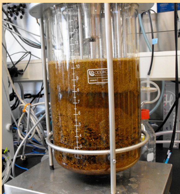
GLBRC Pretreatment Technology. AFEX™-treated corn stover with water before enzymatic hydrolysis, a process that breaks down cellulose polymers into simple sugars using cellulase enzymes. [Image courtesy GLBRC]
