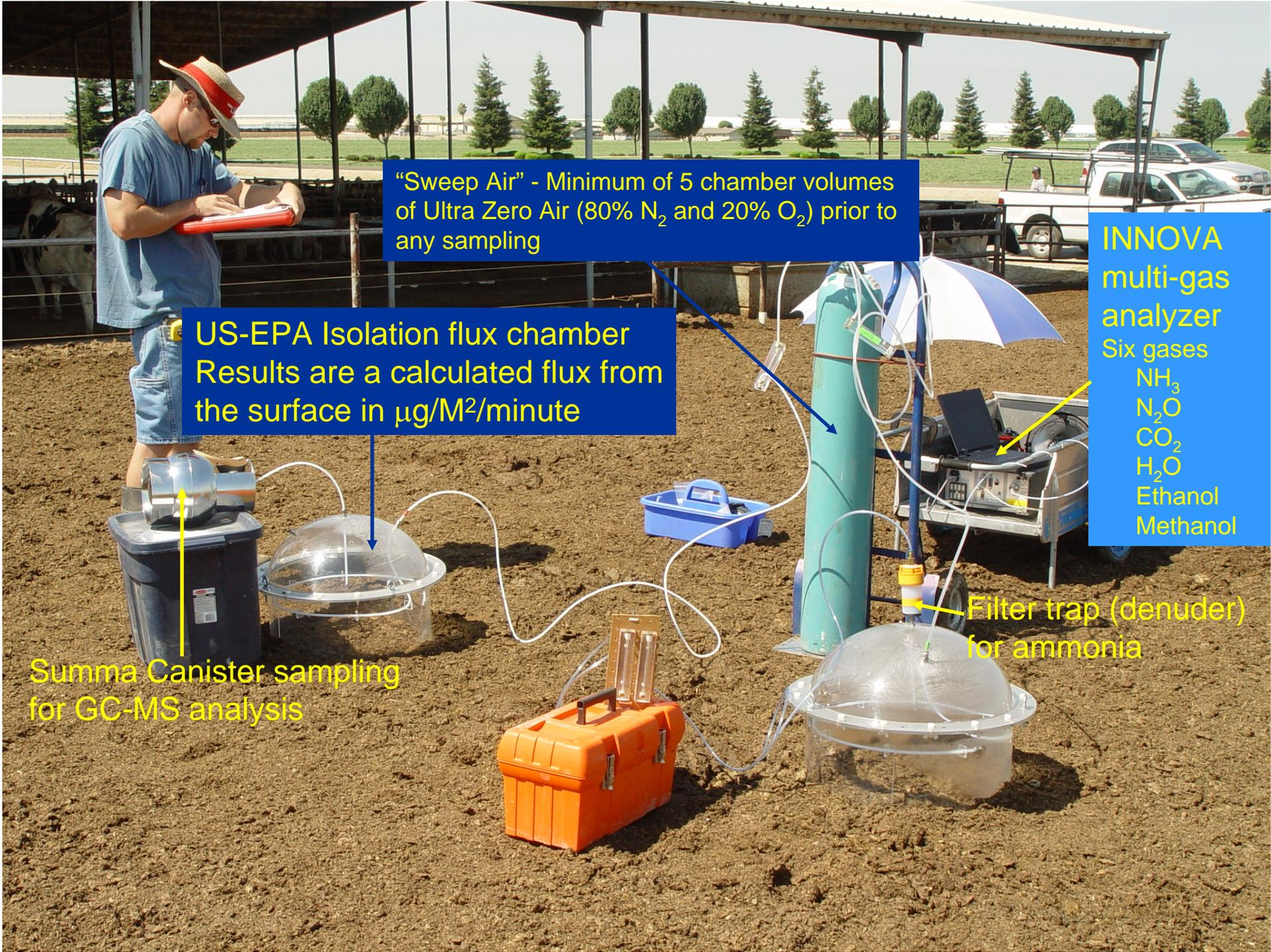
“Sweep Air” - Minimum of 5 chamber volumes of Ultra Zero Air (80% N<sub>2</sub> and 20% O<sub>2</sub>) prior to any sampling
