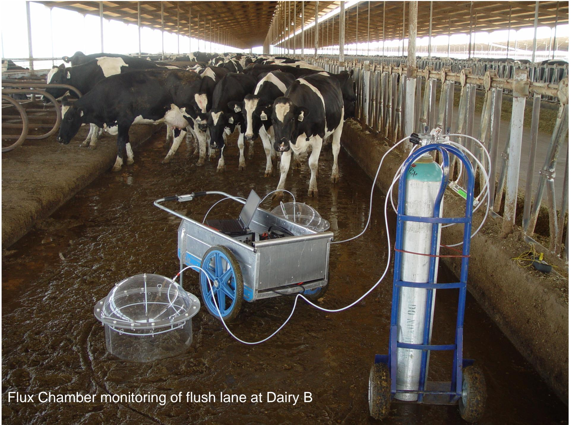
Flux Chamber monitoring of flush lane at Dairy B
