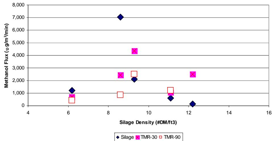
Guidelines for silage production suggest compaction to a density of 10 #/ft<sup>3</sup> or more to reduce diffusion of air into the pile so that yeast fermentation will be inhibited. This fermentation may occur in low compaction piles, resulting in the production and emission of ethanol and, perhaps, other alcohols.
