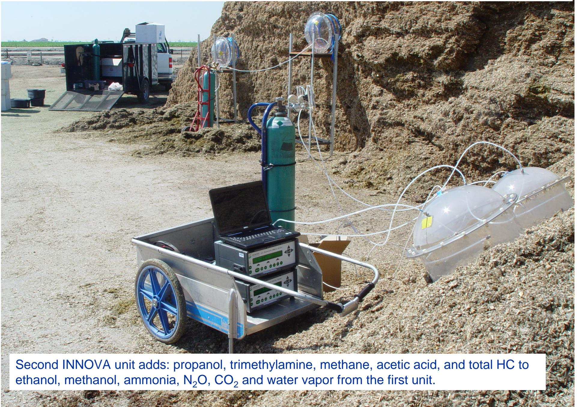
Second INNOVA unit adds: propanol, trimethylamine, methane, acetic acid, and total HC to ethanol, methanol, ammonia, N<sub>2</sub>O, CO<sub>2</sub> and water vapor from the first unit.
