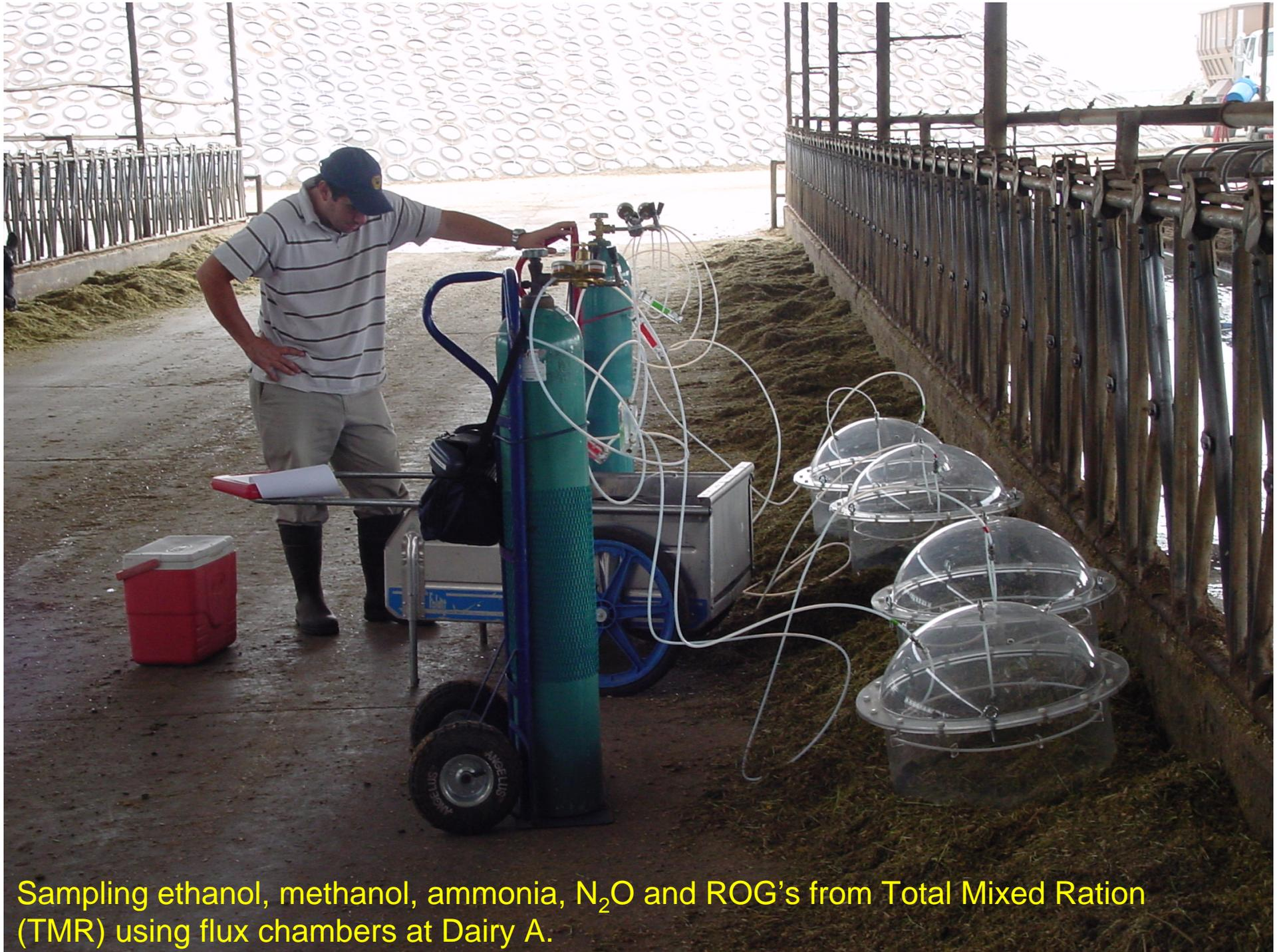
Sampling ethanol, methanol, ammonia,  $N_2O$  and ROG's from Total Mixed Ration (TMR) using flux chambers at Dairy A.
