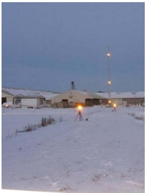
[NH<sub>3</sub>] : 50 ppb–100m (5 ppm-m MDL)
