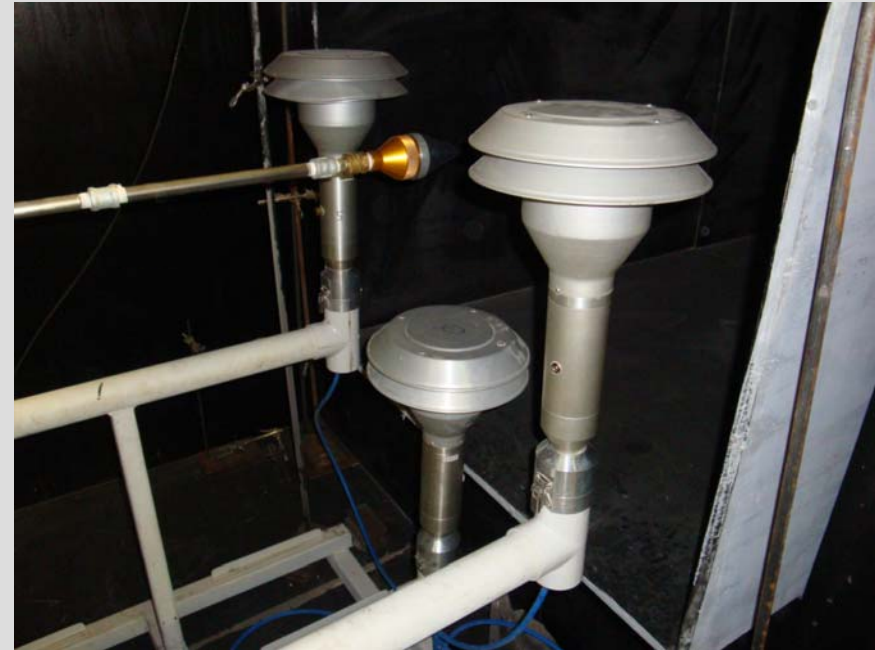
Wind tunnel test section showing arrangement of isokinetic nozzle and PM 10 test samplers
