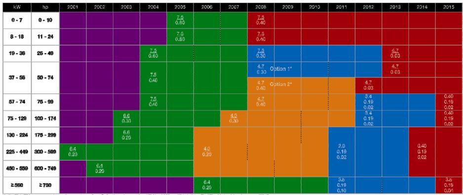
"In the 50 to 75 housepower category there are two options. Option 1 requires a reduced PM level (30 vs.40) but allows Final Tier 4 to be delayed one year (2013).
