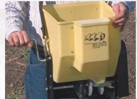
A handheld broadcast seeder.
