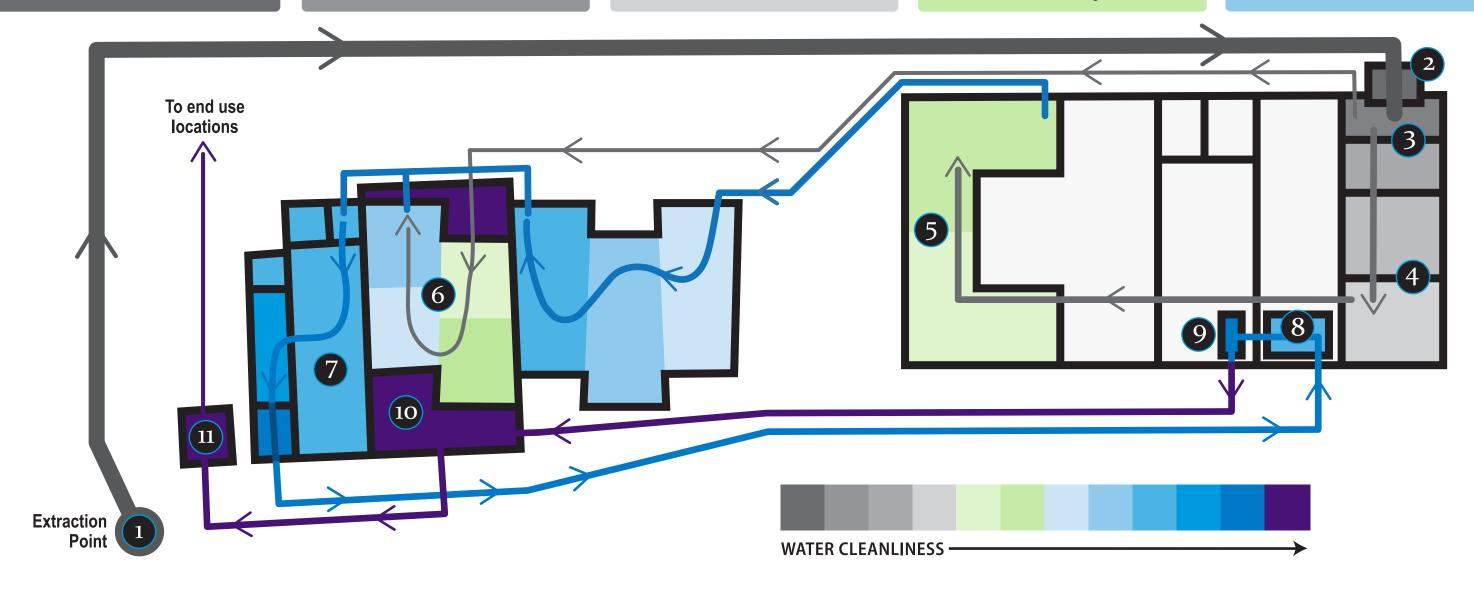
Clarifier Tank. Removal of dissolved phosphorus by use of coagulating elements and gravity. A portion of the solids are sent to the greenhouse to provide ample bacterial communities to begin the treatment process.
