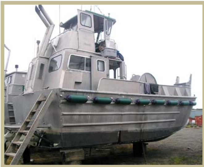
Figure C-14. Twin Jet All American Bowpicker. 32 x 14 ft, or similar vessel. Source: http://alaskaboat.com/boat.php?bid=bp156
