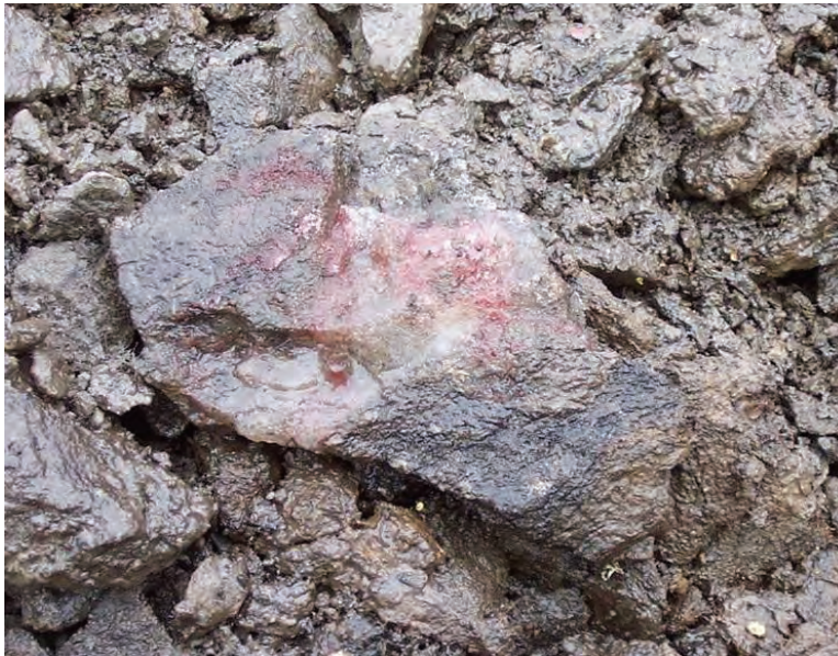
Figure 50. When alpha, alpha-dipyridyl is applied to a soil containing reduced iron, a positive reaction is indicated by a pink or red coloration to the treated area.
