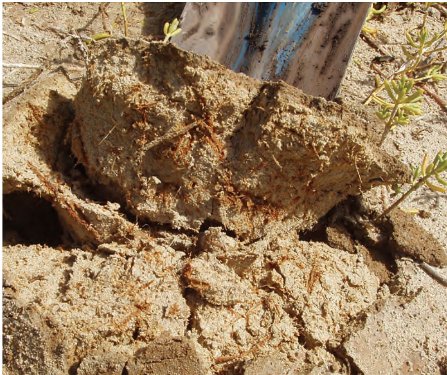
Figure 14. Redox concentrations (orange areas) in loamy fine sand on the Island of O'ahu.
