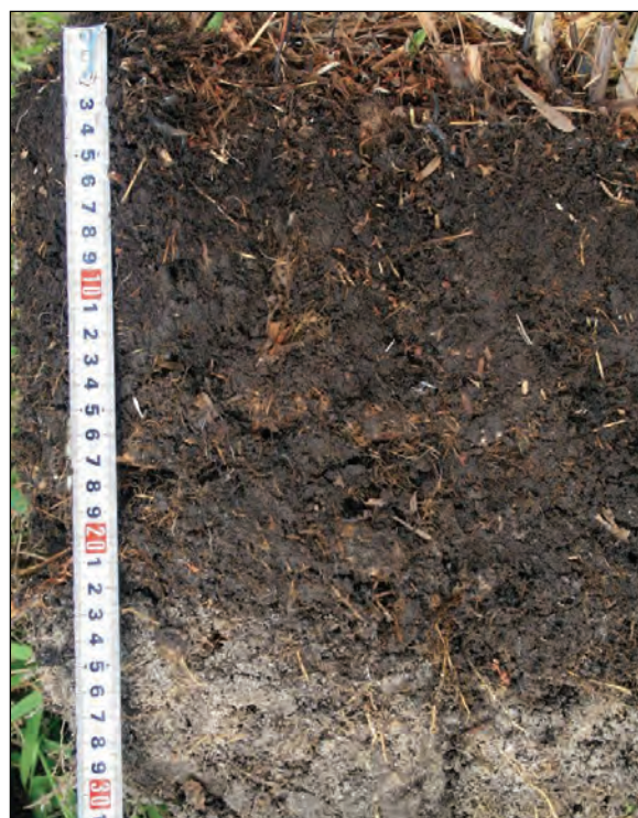
Figure 10. In this soil, the organic surface layer is about 9 in. (23 cm) thick. Scale is in centimeters.
