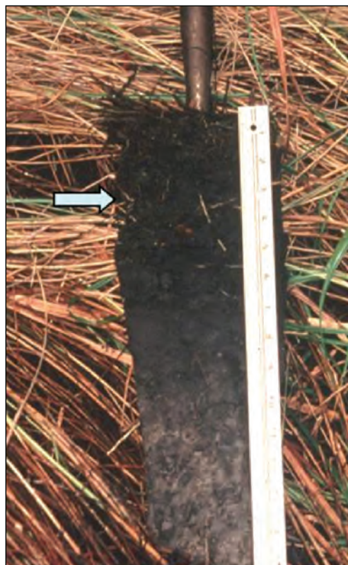
Figure 24. This mucky modified, sandy surface layer is approximately 3 in. (7.5 cm) thick (bottom indicated by the arrow). Scale in inches on the right side of ruler.
