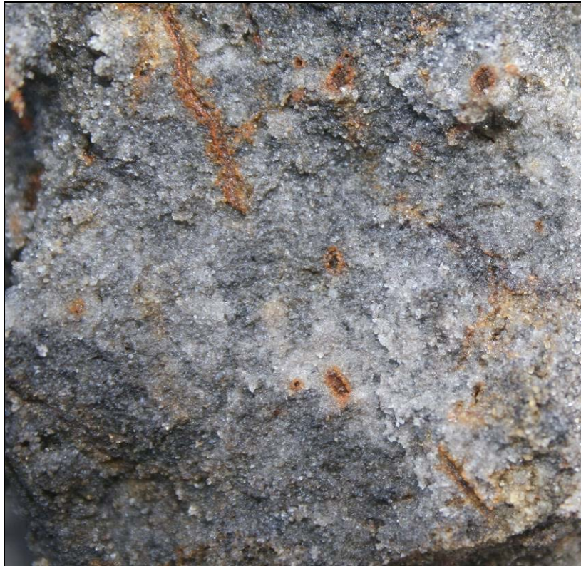
Figure 16. Redox concentrations (orange areas) in sandy soil material.
