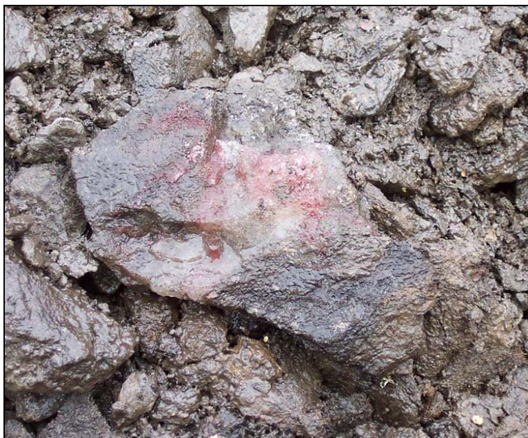
Figure 42. When alpha, alpha-dipyridyl is applied to a soil containing reduced iron, a positive reaction is indicated by a pink or red coloration to the treated area.
