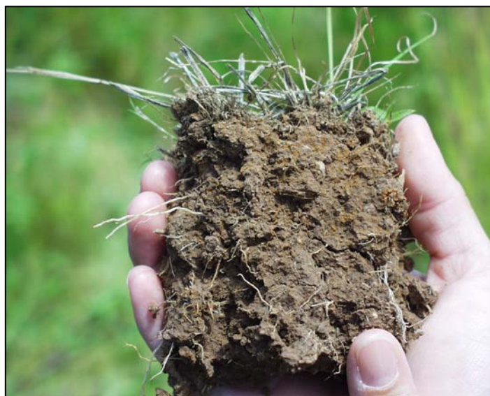
Figure 20. In this example, the layer of redox concentrations begins at the soil surface and is slightly more than 2 in. (5 cm) thick.
