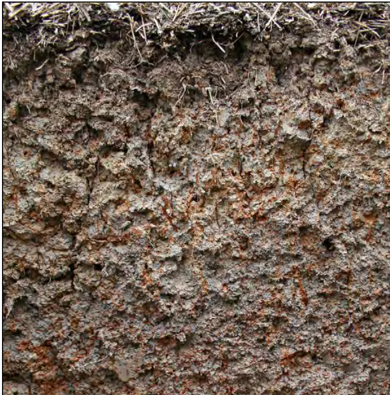
Figure 23. Example of indicator F3 (Depleted Matrix), in which redox concentrations extend nearly to the surface.
