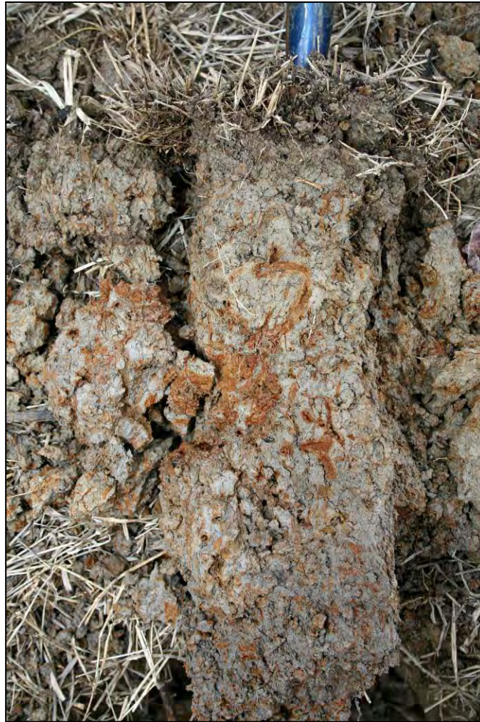
Figure 24. This soil has a depleted matrix with redox concentrations in a low-chroma matrix.
