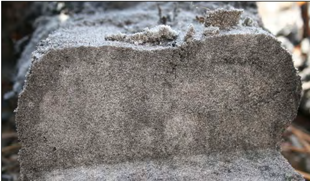
Figure 18. A diffuse, splotchy pattern of stripped and unstripped areas is revealed in this horizontal slice through a sandy soil.
