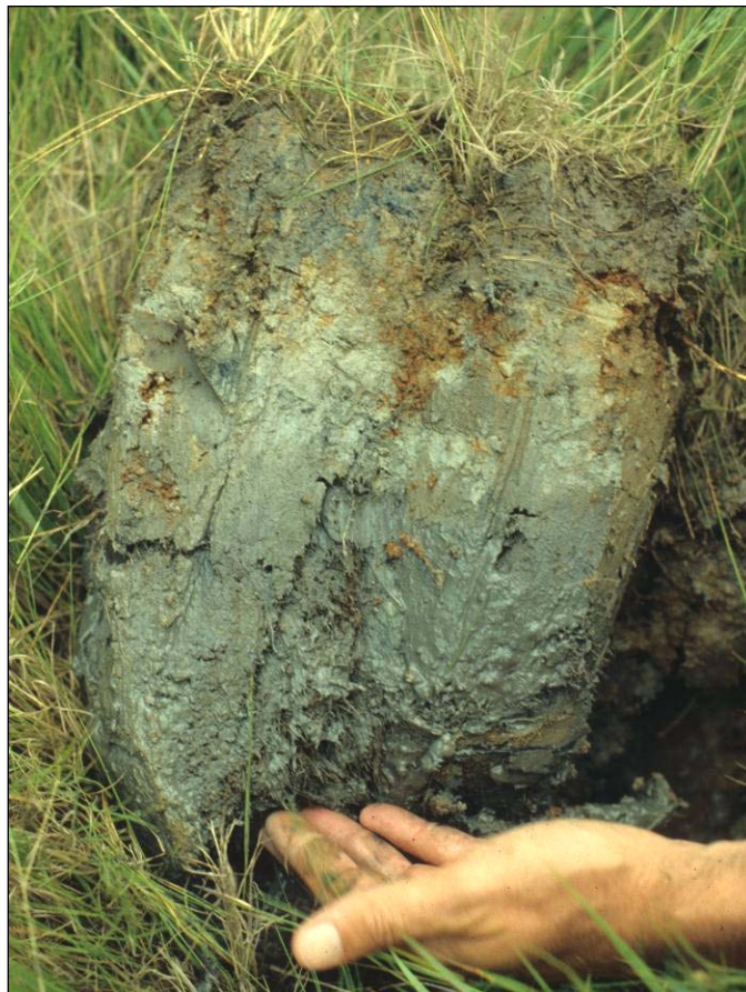
Figure 19. This soil has a gleyed matrix in the lowest layer, starting about 7 in. (18 cm) from the soil surface. The layer above the gleyed matrix has a depleted matrix.
