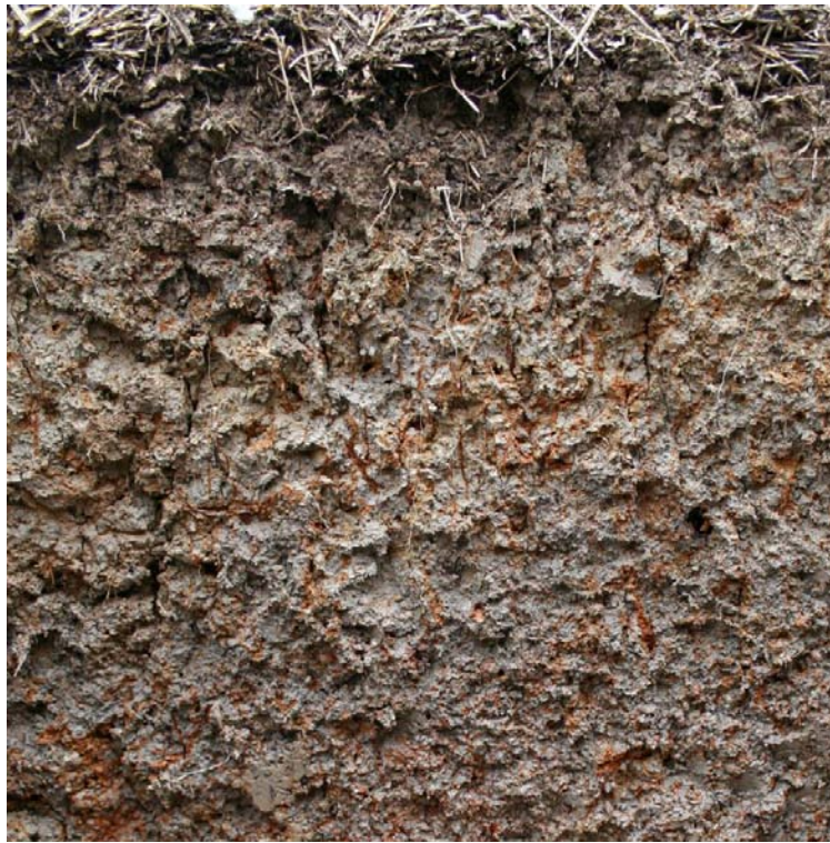
Figure 21. Example of indicator F3 (Depleted Matrix), in which redox concentrations extend nearly to the surface.
