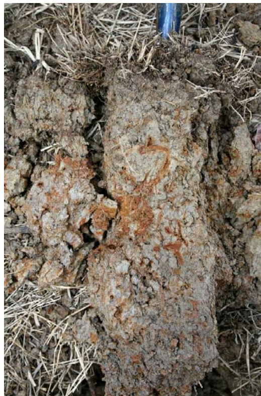
Figure 22. This soil has a depleted matrix with redox concentrations in a low-chroma matrix.
