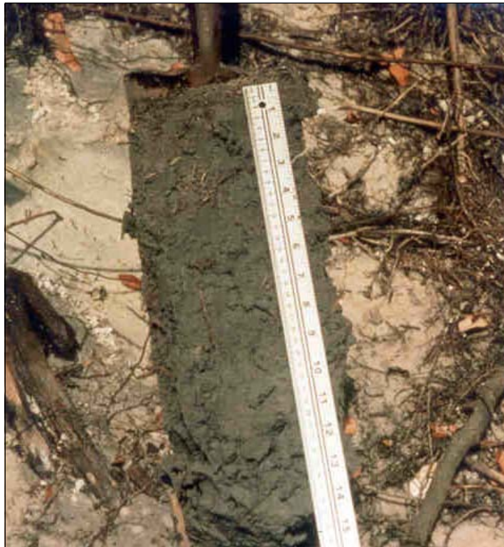
Figure 15. In this example, the gleyed matrix begins at the soil surface.
