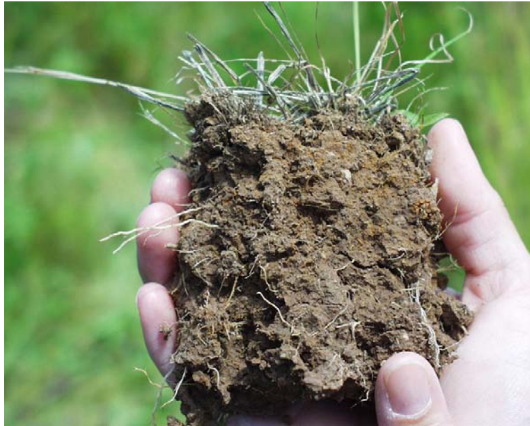
Figure 25. In this example, the layer of redox concentrations begins at the soil surface and is slightly more than 2 in. (5 cm) thick.
