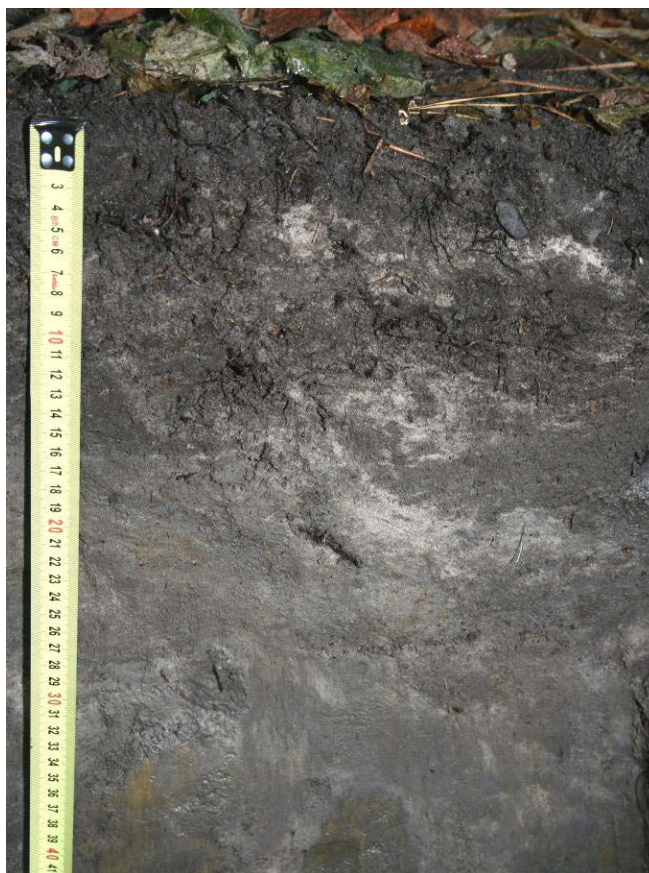
Figure 24. Redox depletions (lighter colored areas) are scattered within the darker matrix. Scale is in centimeters.
