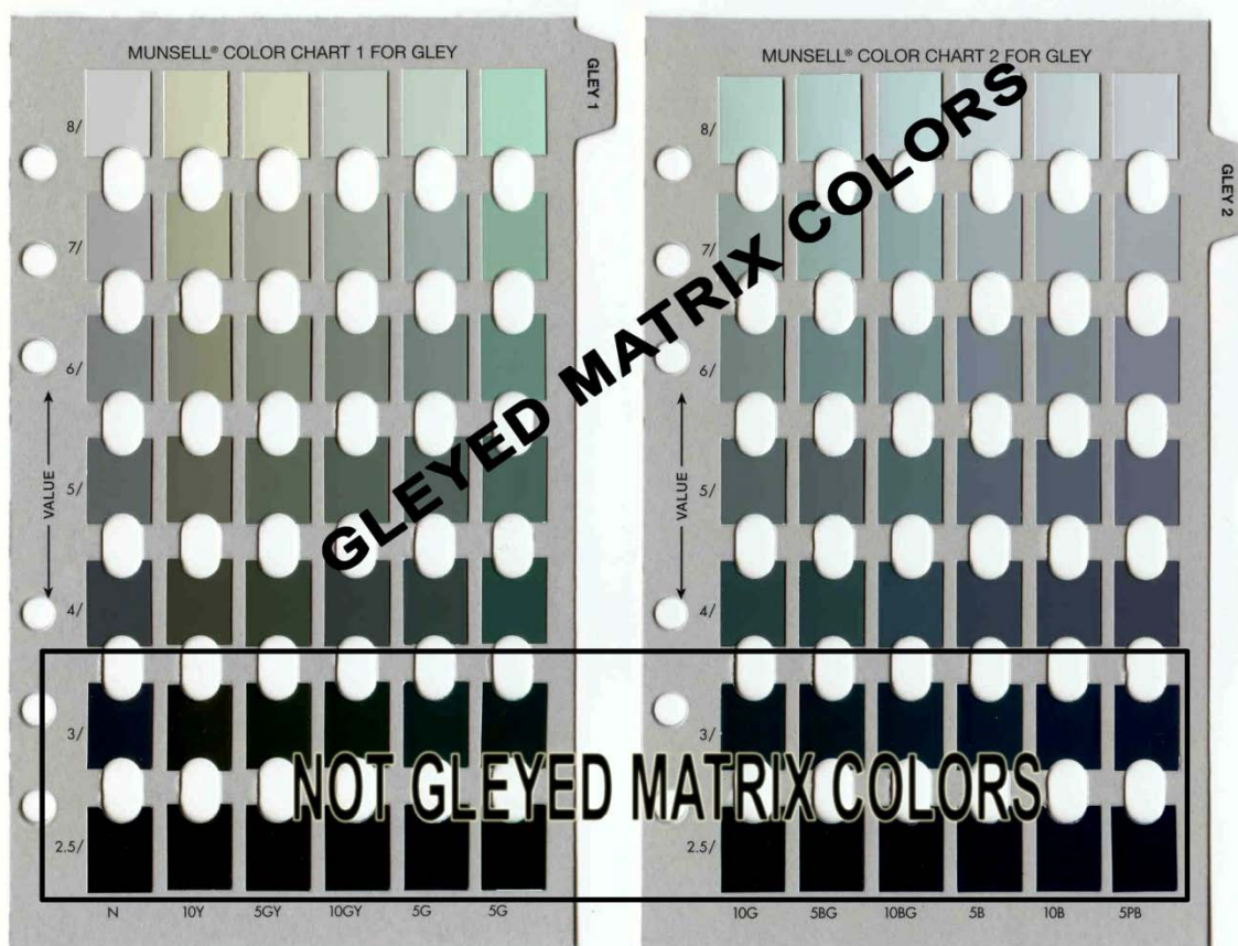
Figure A2. For hydric soil determinations, a gleyed matrix has the hues and chroma identified in this illustration with a value of 4 or more. Due to inaccurate color reproduction, do not use this page to determine soil colors in the field. Background image from the Munsell Soil Color Charts reprinted courtesy of Munsell Color Services Lab, a part of X-Rite, Inc. (Gretag/Macbeth 2000).
