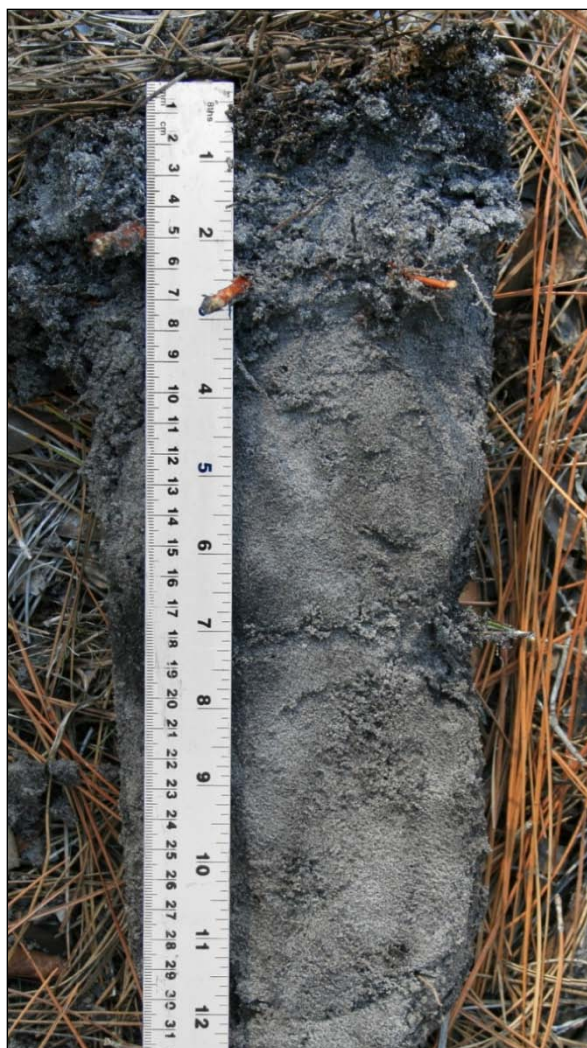
Figure 17. Stripped areas form a diffuse, splotchy pattern in this hydric sandy soil.
