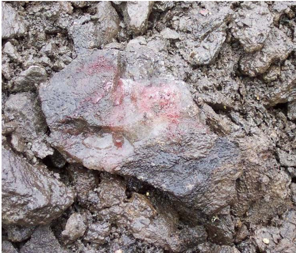
Figure 49. When alpha, alpha-dipyridyl is applied to a soil containing reduced iron, a positive reaction is indicated by a pink or red coloration to the treated area.
