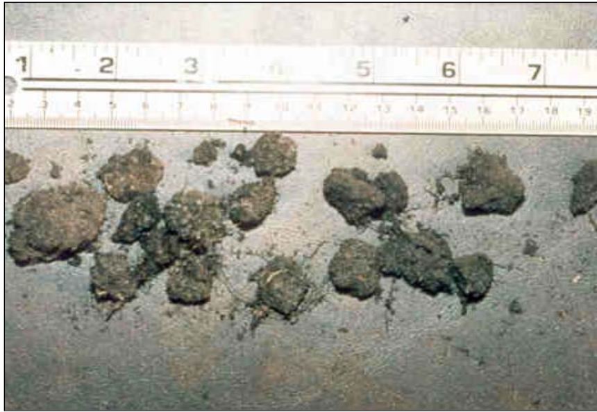
Figure 10. Organic bodies 0.5 to 1 in. (1 to 3 cm) in size. Scale in inches (upper) and centimeters (lower).
