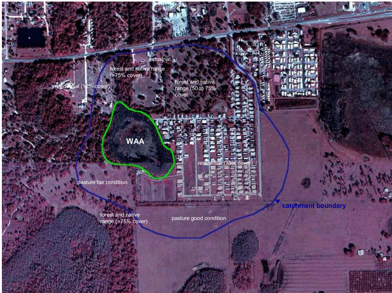
Figure C5. Aerial photograph illustrating examples of some of the cover types found within the catchment of a wetland
