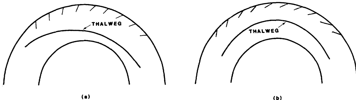
FIGURE 46. COMPARISON OF THALWEG POSITIONS PRODUCED BY SPURS ANGLED AT (A) 120 DEGREE, AND (B) 150 DEGREES.
