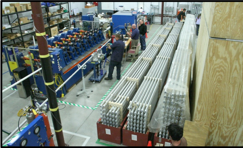
Toroidal field conductor jacketing at High Performance Magnetics (Tallahassee, FL)
