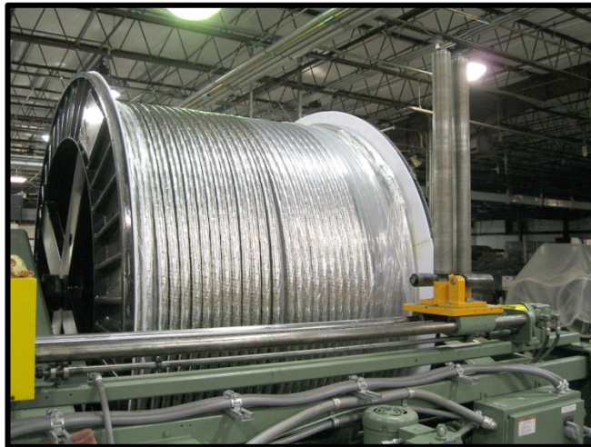
Toroidal field cable produced at New England Wire Technologies (Lisbon, NH)
