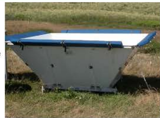
915 MHz phased array wind profiler
