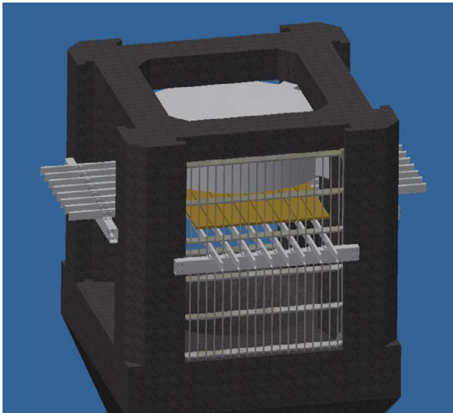
Figure 5. The bulkhead (shown in grey at top) is damaged and must be removed. Aluminum bars would be placed through the intake structure to support platforms to enable workers to remove the bulkhead as well as to prevent materials from falling into the intake structure during removal. After removal is complete, the aluminum bars would be attached to the top of the intake structure to act as a trash rack during reservoir operation.
