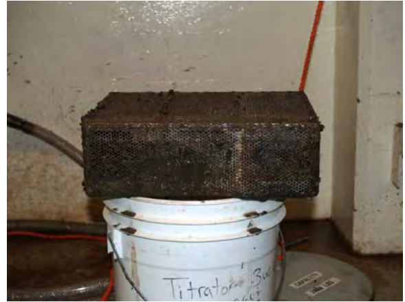
Figure 8: Stainless Steel Bioassay Cage from Bypass System
