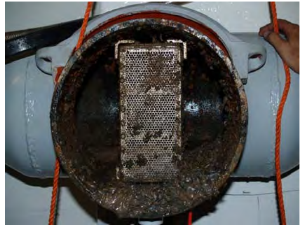
Figure 9: Stainless Steel Bioassay Cage in the Bypass
