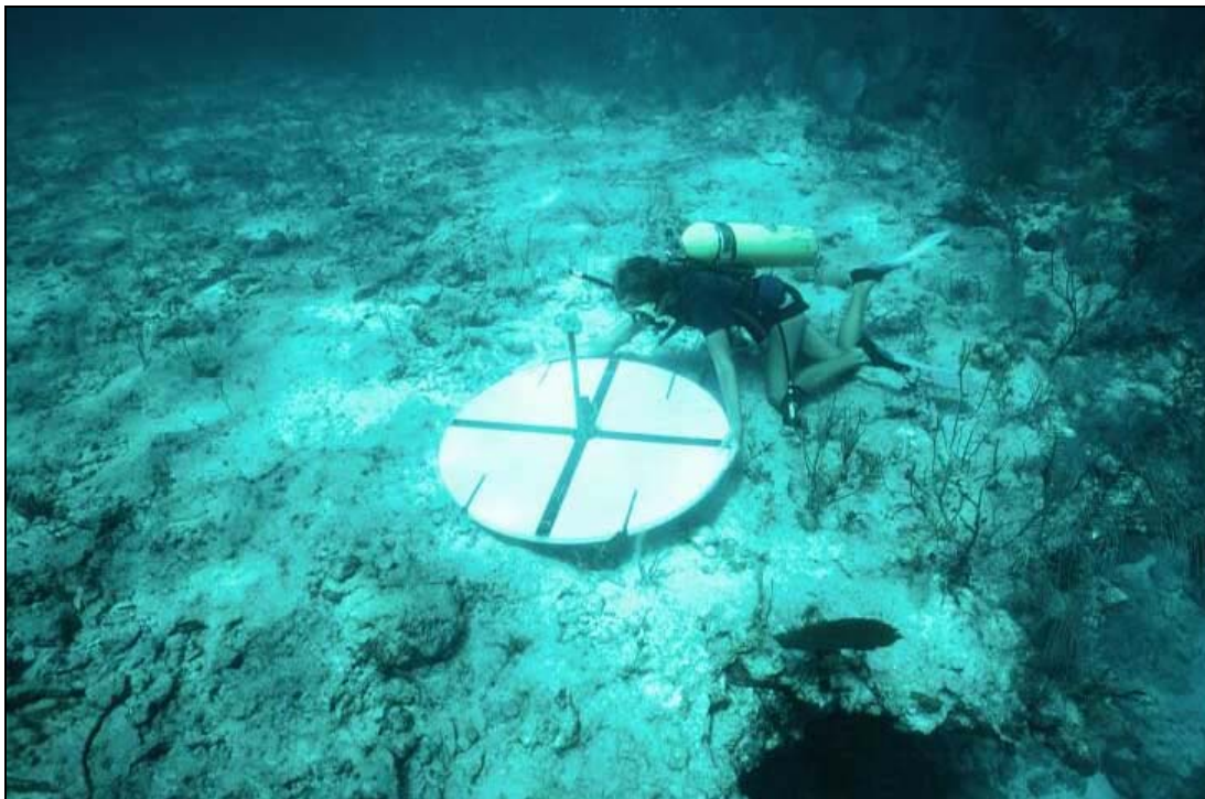
Figure 4. Diver installing 1 m diameter reference marker in the “parking lot” for geo-referencing aerial photography (photo credit: Harold Hudson).
