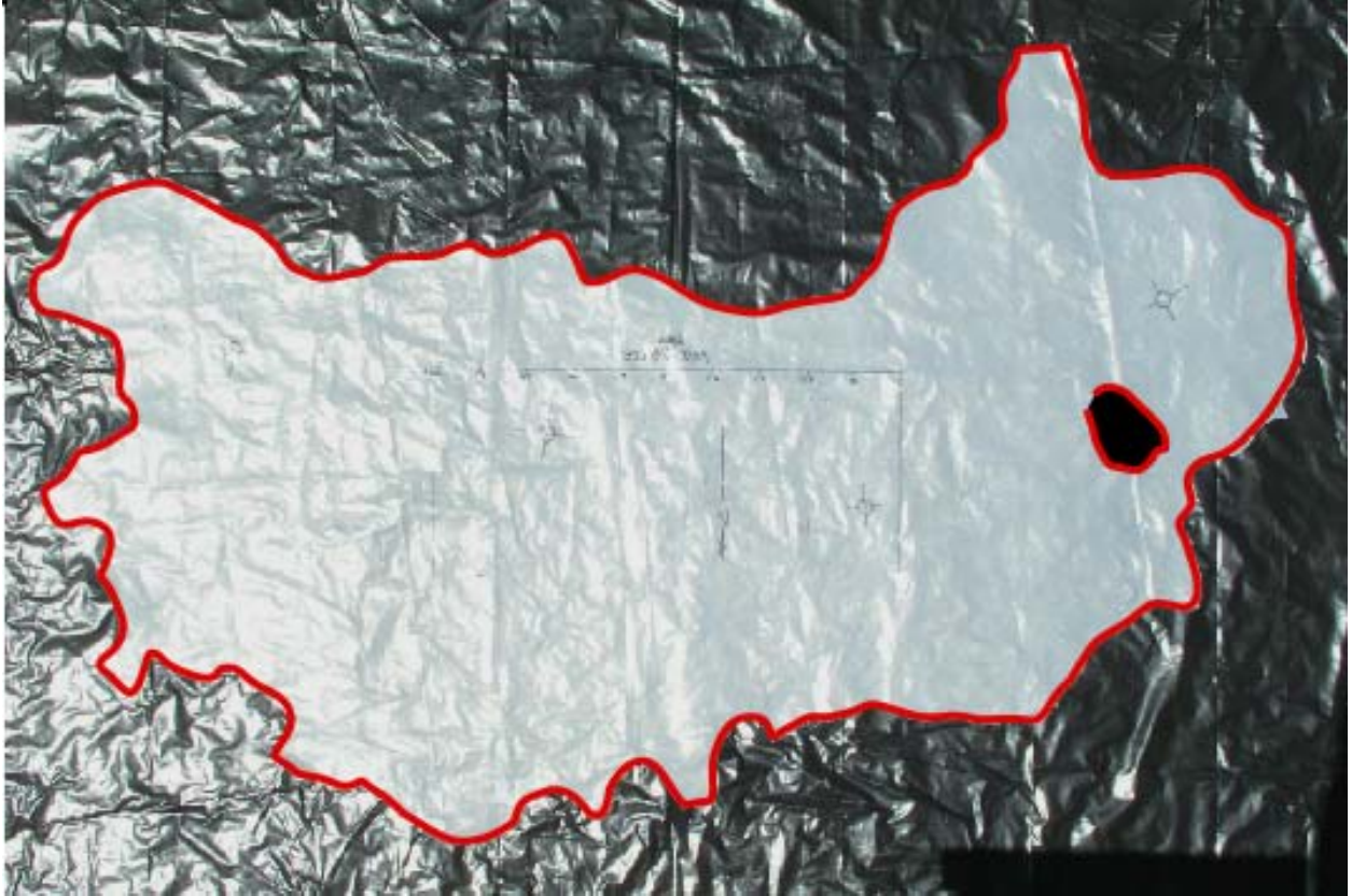
Figure 9. Outline (in red) of the plastic sheet cut to delineate the interface of the concrete surface and live coral tissue along the rim of the coral colony.
