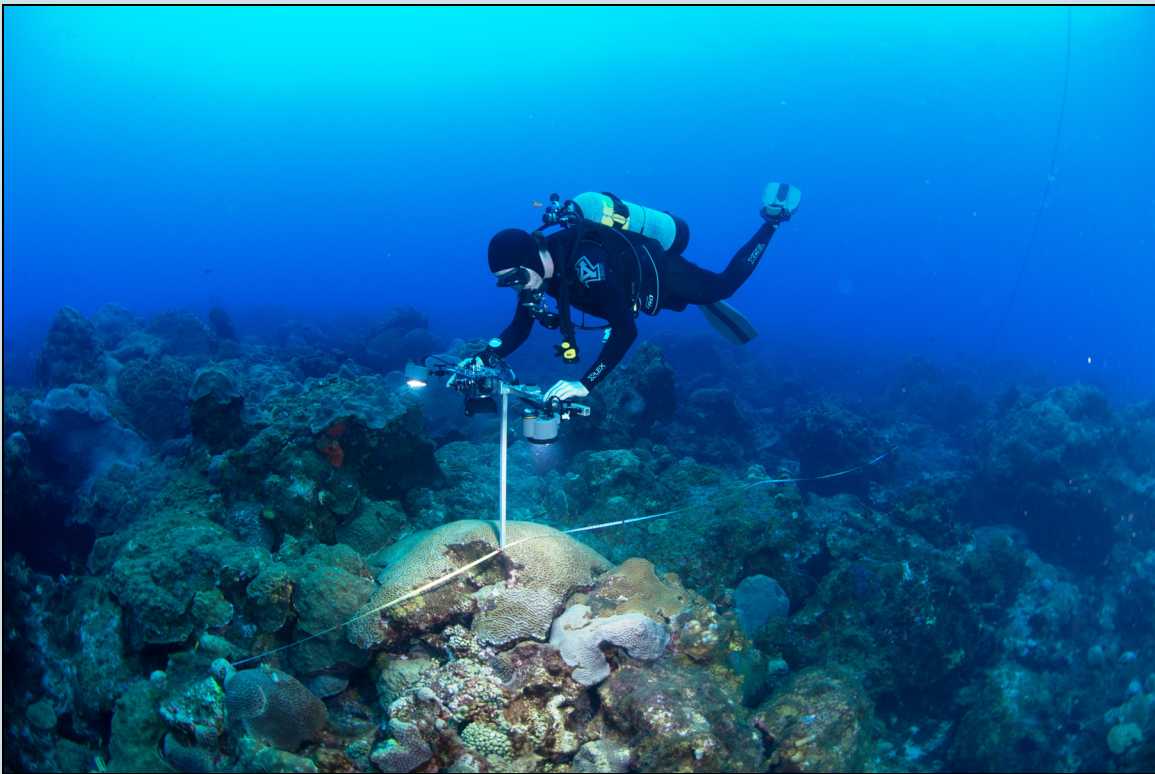
NOAA diver, Ryan Eckert, with camera and strobes mounted on aluminum t-frame taking random transect photographs at East Flower Garden Bank.
