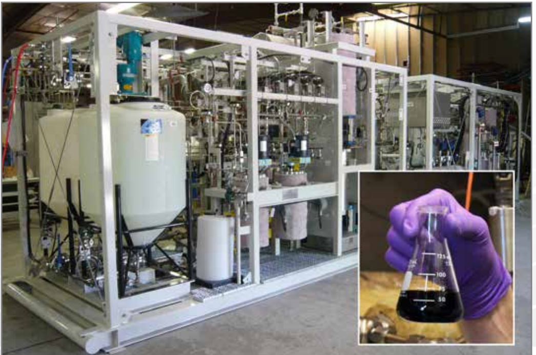
A new hydrothermal process uses heat and pressure to chemically and physically change algae into biocrude in a matter of minutes.
