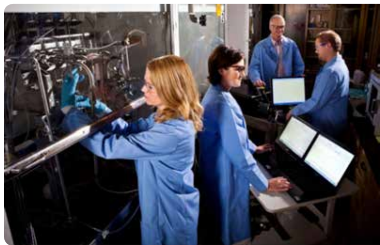
RPL staff collect real-time spectroscopic data on a flow-through solvent-extraction system for research related to nuclear fuel reprocessing.
