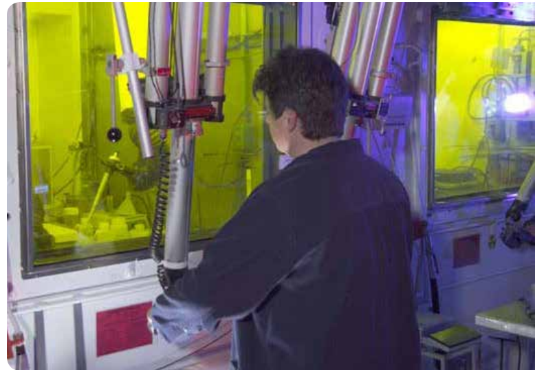
Researchers at Pacific Northwest National Laboratory conduct analytical research on nuclear materials using hot cells that shield the researcher from the radiation.
