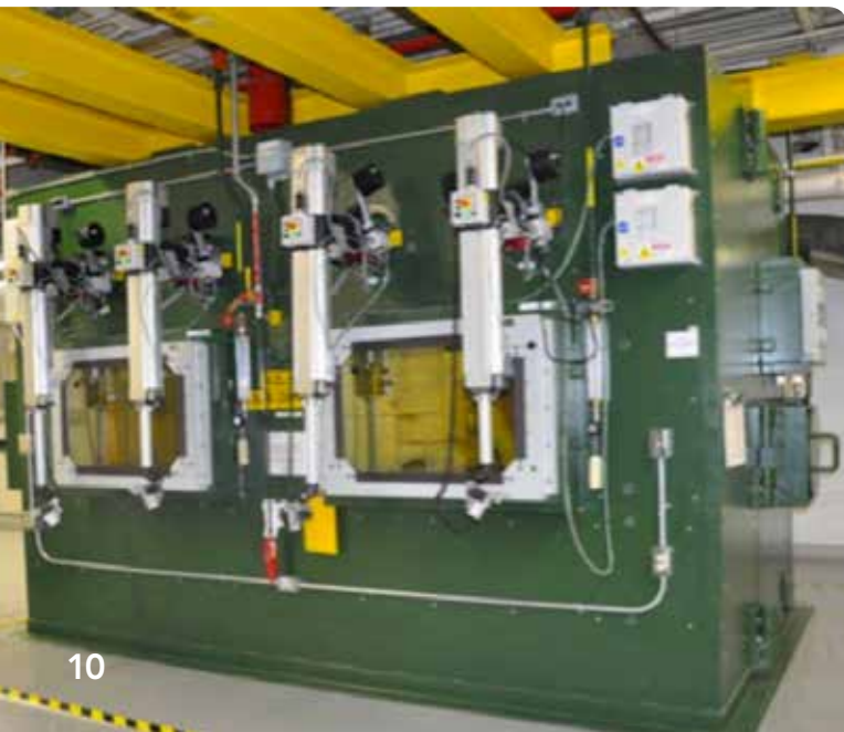
Material examination hot cells housed in the RPL.
