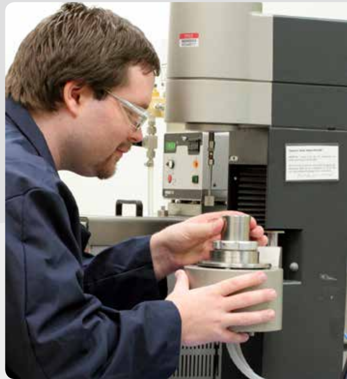
A researcher works with a rheometer to study the fluid-flow properties of complex non-Newtonian media such as solid-liquid suspensions.
