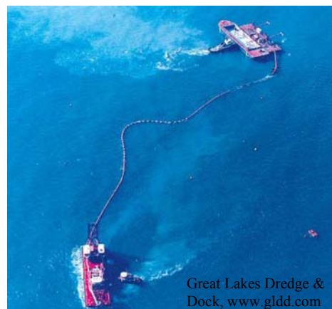
Figure 6. Cutter-Suction Dredge Loading Barges
