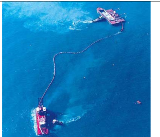
Figure 5. Cutter-Suction Dredge Loading Barges
