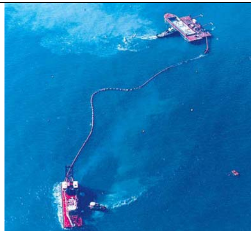
Figure 5. Cutter-Suction Dredge Loading Barges
