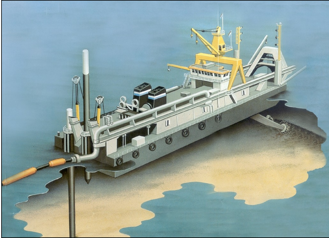
Figure 3. Cutter-Suction Hydraulic Dredge (source: Oilfield Publications Limited, n.d.)
