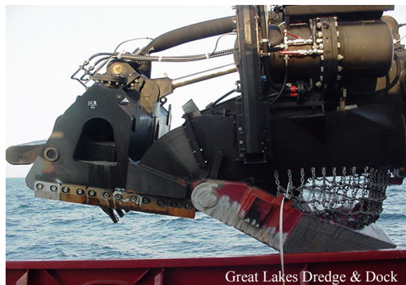
Figure 9. Close-up of a Draghead with a Turtle Deflector Mounted
