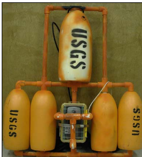
Figure 3. The float used to attach the GPS unit to the trawl.
