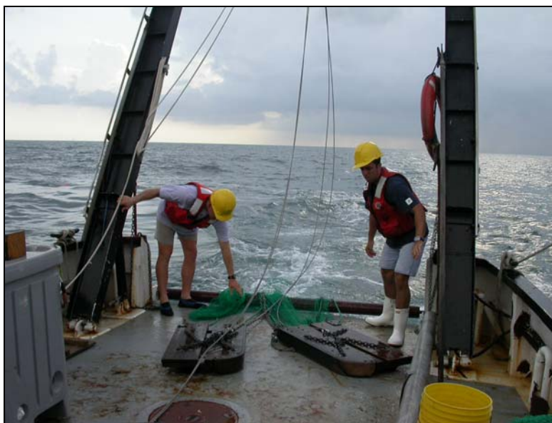
Figure 2. The 6 m otter trawl used for fish sampling.
