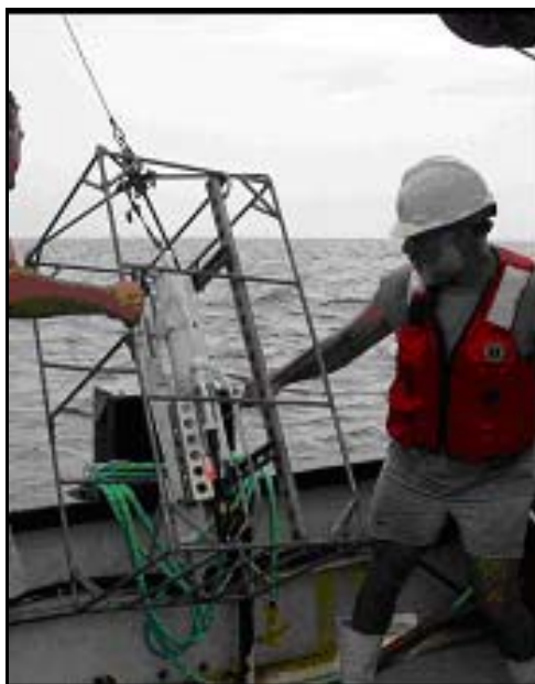
Figure 5. Seabird CTD Deployment, in a custom protective cage for water parameter measurements.
