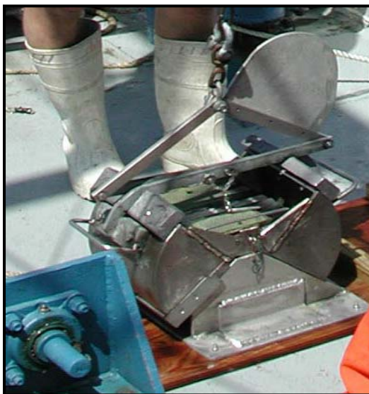
Figure 6. The custom box grab (K. Sulak design) used for sediment collection.
