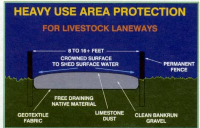
Figure 15 Where the native soils in a laneway cannot support constant heavy traffic, one improvement option is to create a firm layered foundation of successively smaller aggregate, placing it on geotextile material at the bottom of a shallow excavation. The final surface must be above normal grade, crowned to shed rain water, and capped with a fine material to avoid stone bruises to feet.
