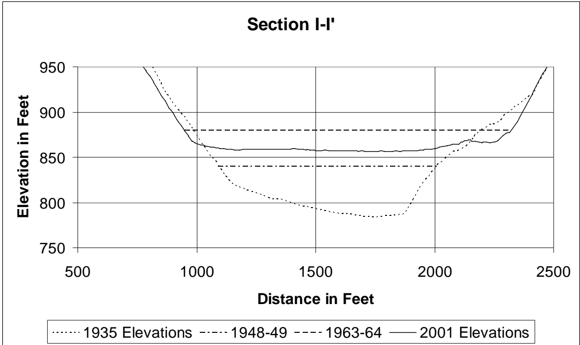
Figure 34- Temple Bar section I-I'
