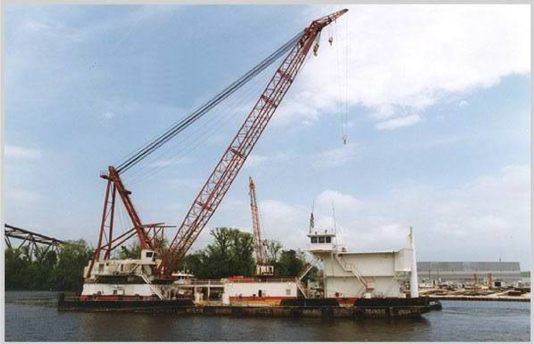
Derrick Barge with Crane
