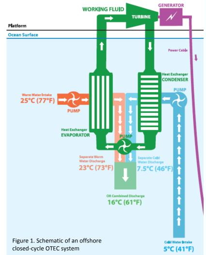
withdraw cold water at a depth of approximately 3300 feet (1000 meters). To accommodate the large cold water flows, the size of the pipe for a 100 MW facility may be approximately 33 feet (10 meters) in diameter. The construction, deployment, and installation of the cold water pipe have remained an engineering challenge.
