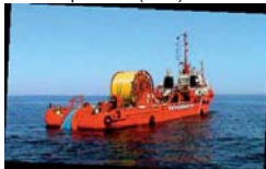
Cable laying ship
