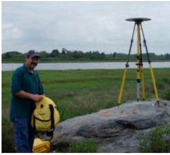
Installing a new United States Geodetic Survey benchmark on Prudence Island.
