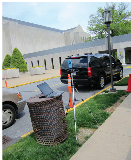
Figure 3. A laptop computer with two Vernier temperature probes and one CO 2 probe was set up in the carpool lane while a time-lapse camera recorded the arrival of cars.
