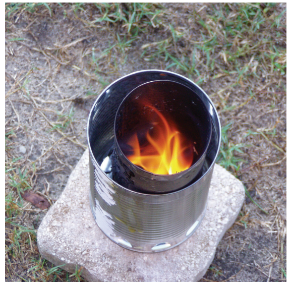
Figure 1. Small student-built top-lift updraft pyrolyzer made from recycled cans. A fire is lit from the top as biomass (in this case pine pellets) is gasified and the volatile gases combust. When pyrolysis is completed, the remaining material is quenched, leaving behind biochar.
