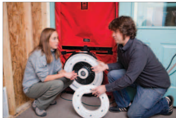
Getting hands-on with a blower door.
