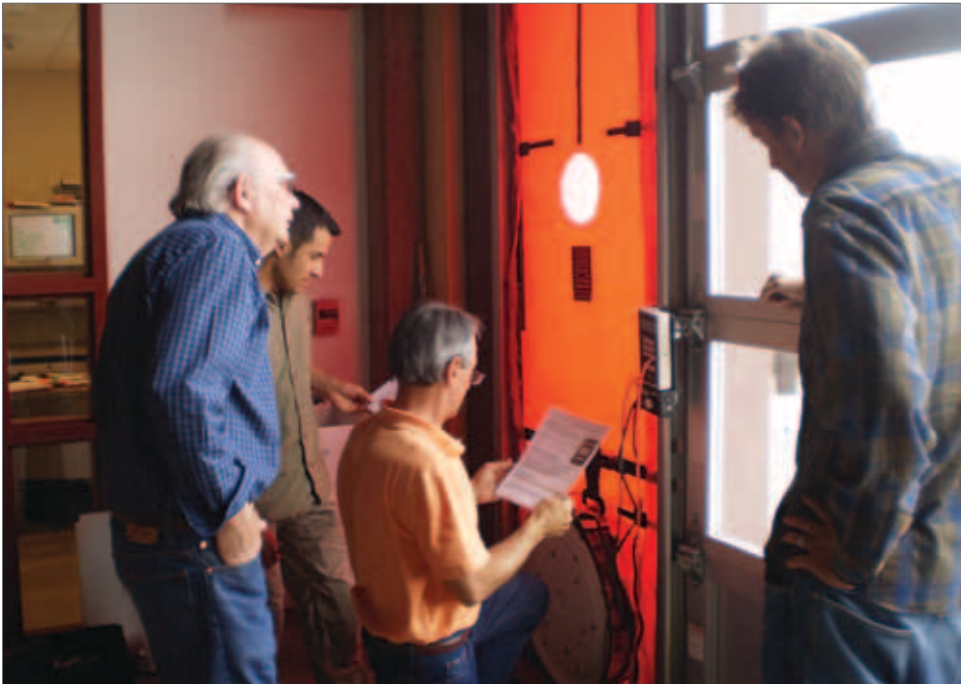
Peer-to-peer learning—figuring out how to program a manometer together.
