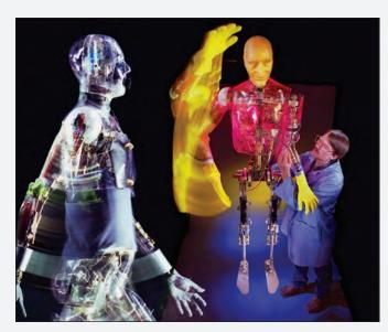
In 1988, engineers at PNNL developed "Manny," the robotic mannequin—that was so humanlike it even sweated—for the U.S. Army to test protective clothing for extreme use conditions.
