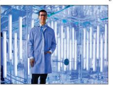
PNNL offers a state-of-the-art Aerosol Test Chamber located in the Atmospheric Measurements Laboratory to study the aerosol lifecycle. The glow, generated by ultraviolet lights, simulates the sun. Data derived from experiments using the chamber will be used for model validation and incorporated into climate models developed by PNNL.
