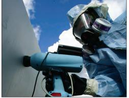
PNNL developed the Acoustic Inspection Device to help identify the contents of sealed containers. For nearly 20 years, PNNL has trained officials from around the world to use this technology and others to help detect materials or components of weapons of mass destruction being shipped across borders.
