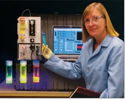
The Biodetection Enabling Analyte Delivery System, or BEADS, developed by PNNL could be used to detect protein signatures including E. coli, salmonella, ricin and other toxins or biological weapons with high specificity and high sensitivity in dirty environments.
