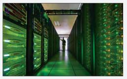
The 3.4 petaflop Cascade supercomputer at EMSL, the Environmental Molecular Sciences Laboratory, is available to researchers around the world. The system's 23,000 Intel processors have 184,000 gigabytes of memory available—about four times as much memory per processor as other supercomputers.
