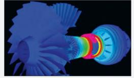
In 2006, PNNL and Advanced Virtual Engine Test Cell Inc. set out to improve computer models that simulate turbine engine performance and could reduce manufacture time. This simulation of a full aircraft jet engine includes all major components. Color indicates pressure changes in the engine and temperature changes in the combustor.
