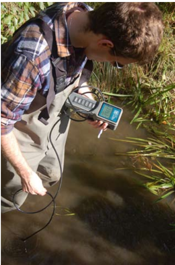
A research intern takes water quality measurements in a local brook using a handheld datalogger.
