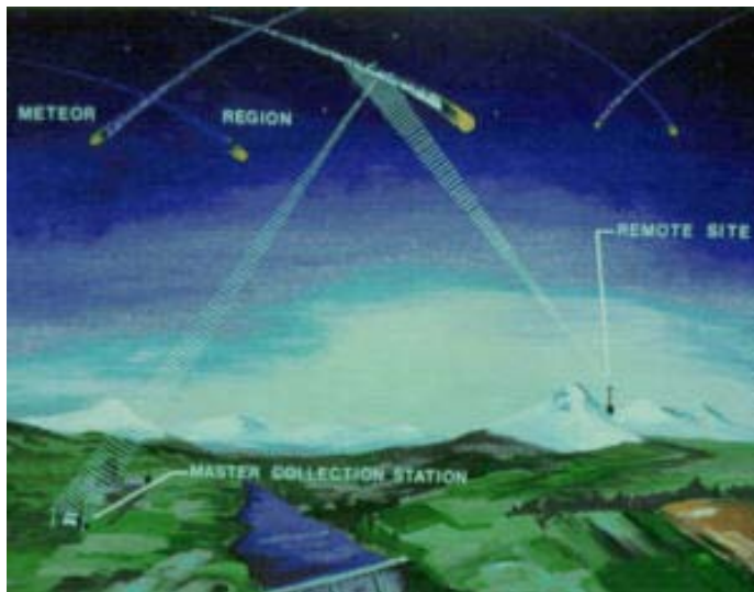
Artist's schematic of meteor burst technology at work.
