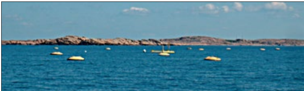
Figure 4.1. Wave energy converters (WECs) and environmental buoys deployed at the Lysekil Research Site. These WECs and buoys have been used for researching potential effects on benthic communities, reefing, and colonization. Underwater noise from a single WEC has also been investigated. (Figure from Haikonen 2014).
