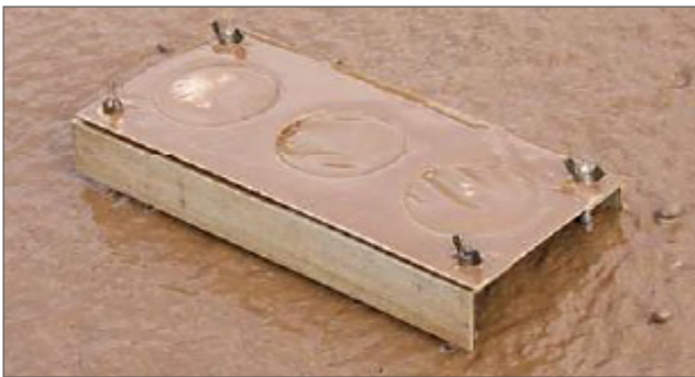
Figure 5.1 Example of sediment trap filters used from Starrs Point, in the Bay of Fundy. Sediment traps are placed on the surface of intertidal mud flats and measure sediment deposition under different tidal cycles (from van Proosdij et al. 2013).
