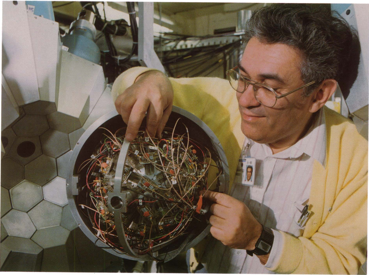
Figure 46: The “Dwarf Ball” charged-particle detector developed at Washington University. It is shrunk in size to fit inside a 4\pi\gamma -detector array such as shown in the left part of the figure. The “ball” consists of 104 elements of scintillator sandwiches and can measure the charge number and energy of reaction products up to Z = 20 with single-charge resolution. The fine segmentation allows detection of a large number of simultaneously emitted fragments and determination of their distribution in space.
