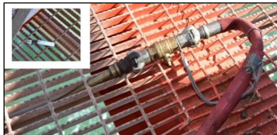
Figure 28 - Hose Nozzle and Handle (November 21, 2014)
