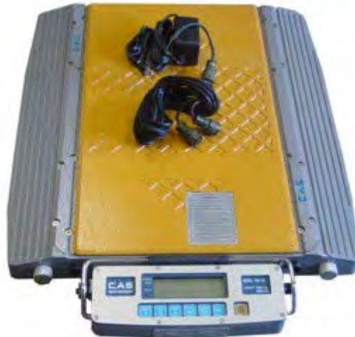
Figure 44. A wheel pad (photo credit: http://www.onboardscales.com/wheel-weigher-truck-1.htm )
