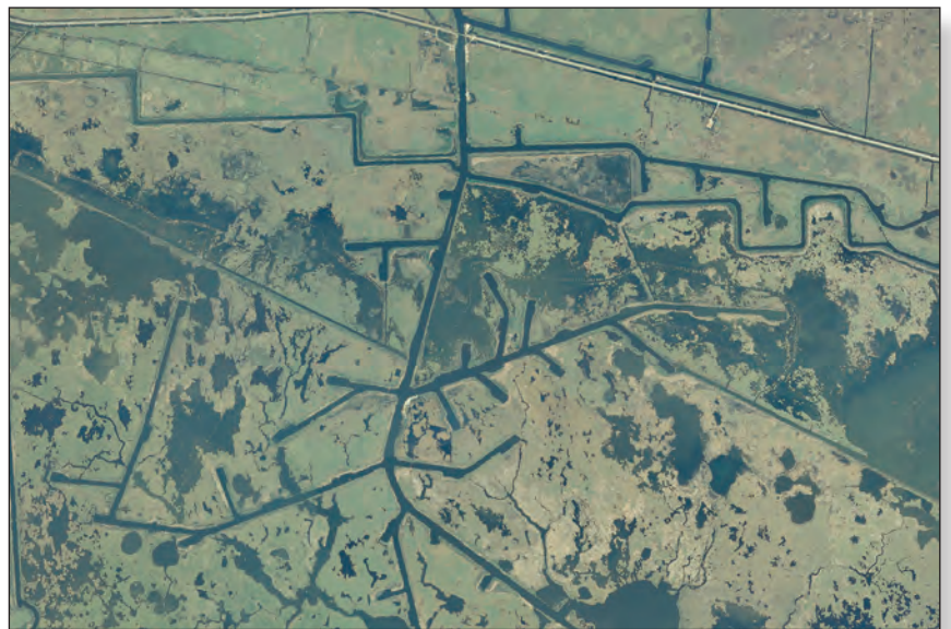
Figure 28. Oil and gas field development located in estuarine (salt-marsh) wetlands of southern Louisiana. Such modifications have increased the vulnerability of these wetlands to climate related change (Twilley 2007) and the cumulative impacts have contributed to relative sea level rise, marsh fragmentation, and subsidence.
