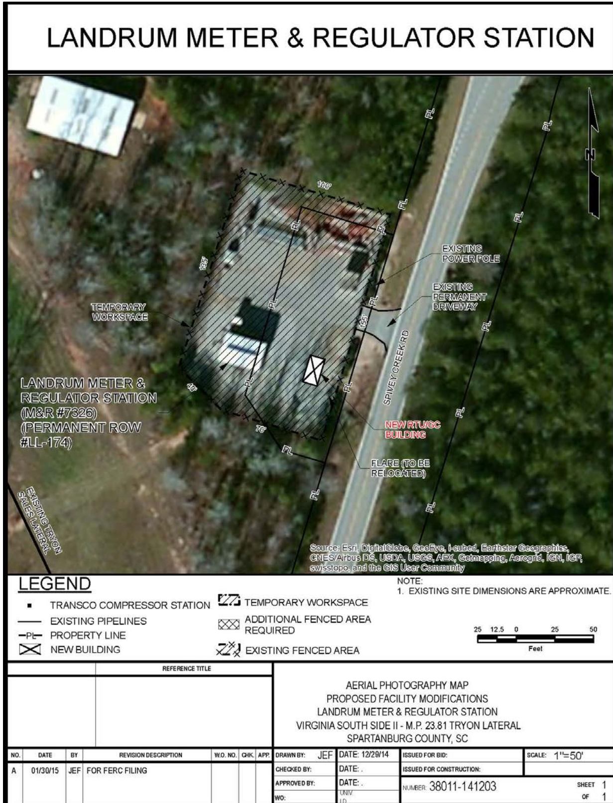
Figure A- 9. Proposed modifications at Landrum Meter and Regulator Station (Spartanburg County, South Carolina)
