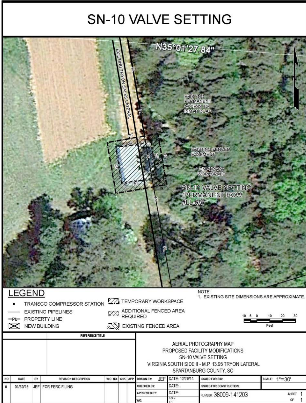
Figure A- 11. Proposed modifications at SN-10 valve setting (Spartanburg County, South Carolina)
